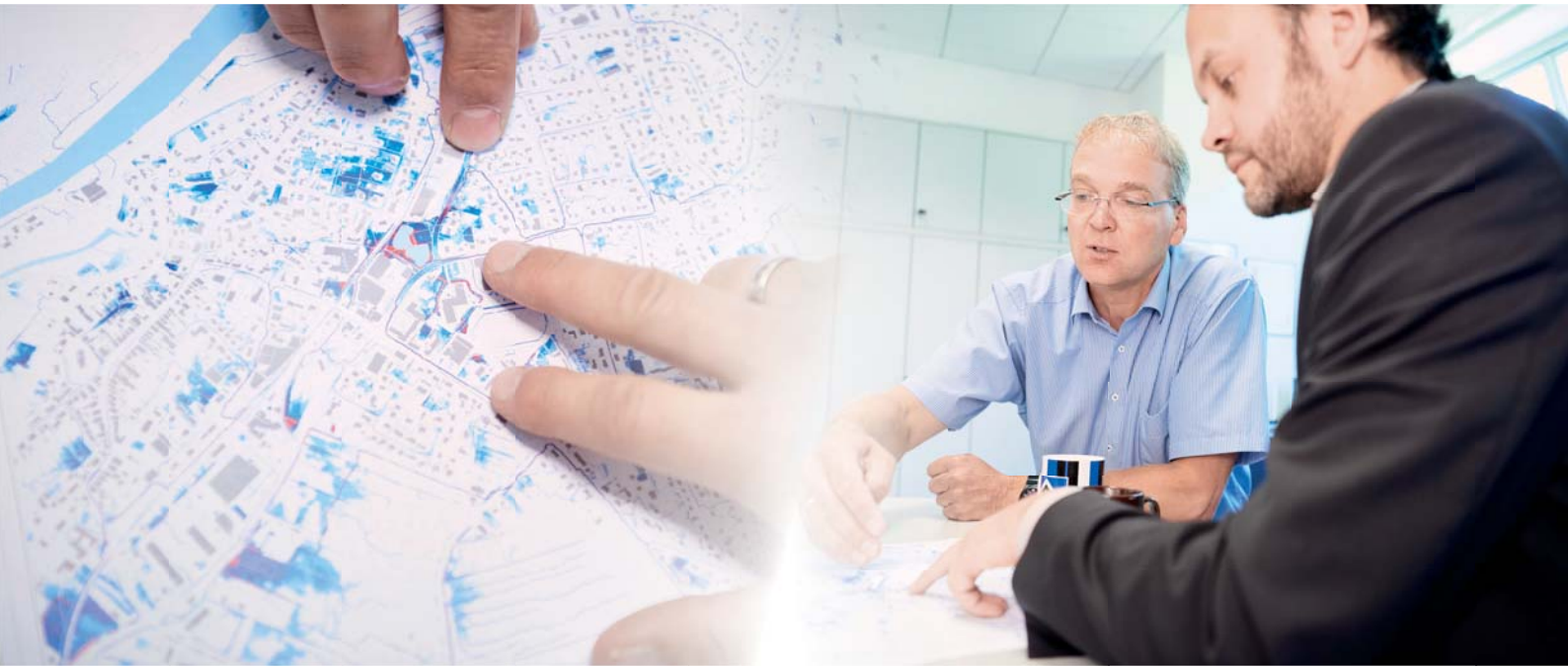
The map of Bleckede shows the simulation of a heavy rain event. The areas in blue and red depict the areas that would be flooded.
